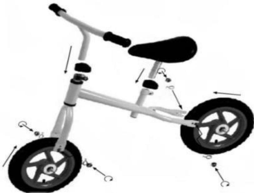
This bike has two styles. The frame can be rotated upside down (for bigger children). It's easy to change the frame style by only needing to loosen the caliper with the allen key .
